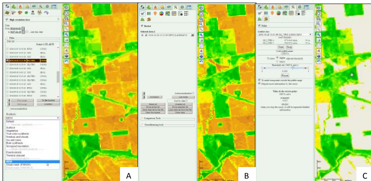
Fig.70 Palette tool allows to color the data only above (or below) a prescribed threshold. It is usable for detecting areas with a certain NDVI values at the satellite images in VEGA-GEOGLAM.
